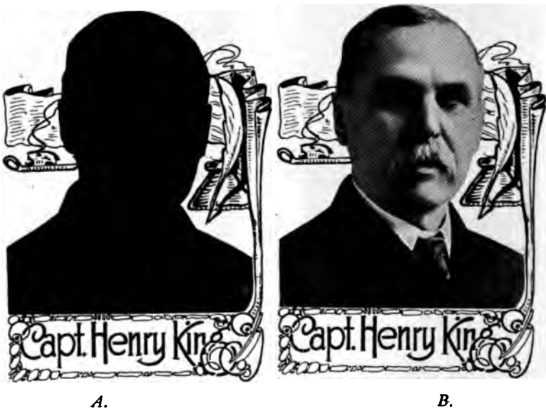
Fig. 23—(A) Pen decoration with silhouette for halftone insert. (B) A combination line and halftone picture (85-line screen).
